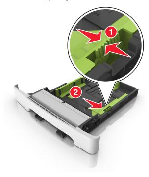
**Note:** Use the paper size indicators on the bottom of the tray to help position the guides.
