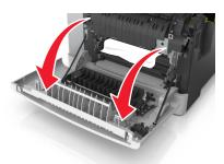
**a** If there is a jammed paper under the fuser, then firmly grasp the paper on each side, and then gently pull it out.
