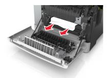
**b** Pull the green lever to open the fuser cover.
