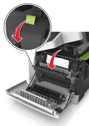
**c** If there is a jammed paper in the fuser, then hold down the fuser cover, and then remove the paper.
