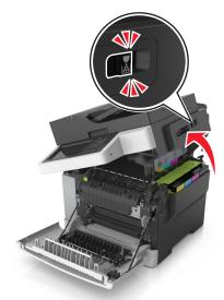
**3** Pull the green lever to open the fuser cover.
