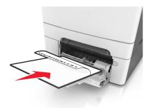
• Load envelopes with the flap side up and against the right side of the paper guide.
