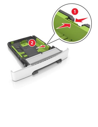
**3** Squeeze, and then slide the length guide tab to the correct position for the paper you are loading.
