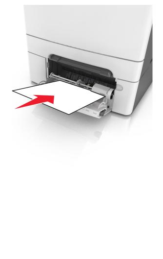
**4** Slide the paper guide until it lightly rests against the edge of the paper stack.
