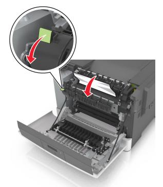
**3** Hold down the fuser cover, and then remove the jammed paper.
