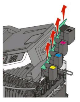
Remove the toner cartridges by lifting the handles and then gently pulling away from the imaging kit.
