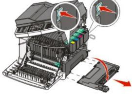
Push in the green touch points on each side of the cartridges to release the side panel, and then remove it.
