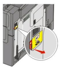
**8** Temporarily connect a USB cable between the computer on the wireless network and the printer.
