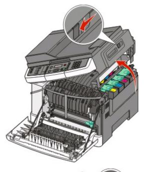
Slide the release latch to the left and lift to open the top
