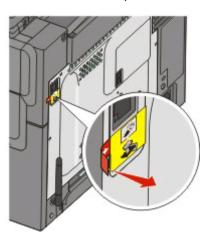
7 Connect the installation cable to a USB port on the computer and the USB port on the back of the printer.
