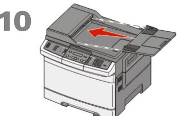
Attach the ADF tray, the exit tray, and the paper bail to the printer as shown.
