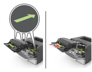
**8** Insert the toner cartridge by aligning the side rails of the cartridge with the arrows on the side rails inside the printer, and then insert the cartridge into the printer.
