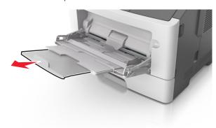
2 Squeeze the tab on the left width guide, and then move the guides for the paper you are loading.
