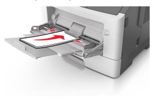
**Warning—Potential Damage:** Never use envelopes with stamps, clasps, snaps, windows, coated linings, or self-stick adhesives. These envelopes may severely damage the printer.
