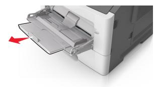
**b** Pull the extender gently so that the multipurpose feeder is fully extended and open.
