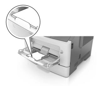
• Load letterhead faceup with the top edge entering the printer first. For two-sided (duplex) printing, load letterhead facedown with the bottom edge of the sheet entering the printer first.
