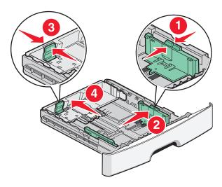
If you are loading a longer size of paper like A4 or legal, squeeze the length guide tab and slide the length guide backwards to the position for the length of paper you are loading. The tray extends backwards as shown.
