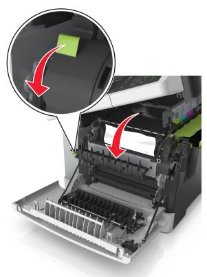
4 Hold down the fuser cover, and then remove the jammed paper.Note: Make sure all paper fragments are removed.
