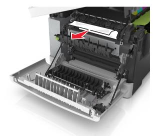
**5** Slide and hold the release latch on the right side of the printer, and then slowly close the top door.
