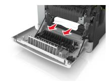
**b** Pull the green lever to open the fuser cover.
