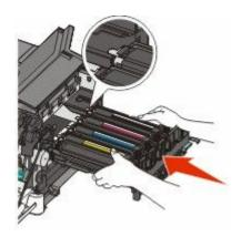
15 Gently, but firmly push the blue levers down until the imaging kit drops into place.
