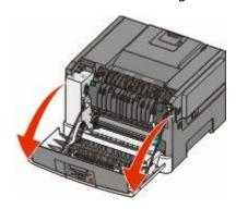
**b** If the jam is visible, remove the jammed paper.
