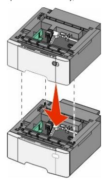
4 Align the printer with the 650-sheet duo drawer, and then lower the printer into place.
