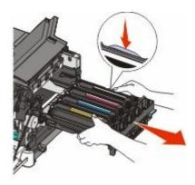
**8** Remove the used developer unit.
