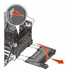
Press the green levers on each side of the waste toner box, and then remove it.
