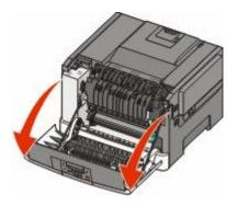
Open the top door by sliding the button forward.
