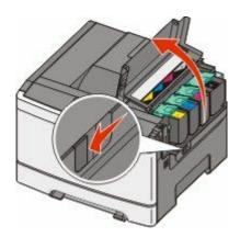
4 Remove the toner cartridge by lifting the handle, and then gently pulling it away from the imaging kit.
