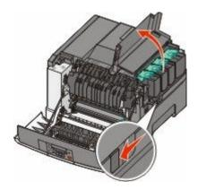
Remove the toner cartridges by lifting the handles and then gently pulling them away from the imaging kit.
