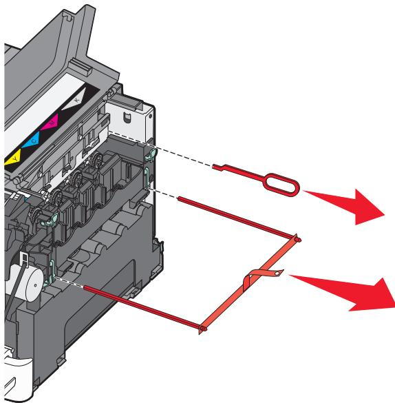
Remove the packing rods and clips.
