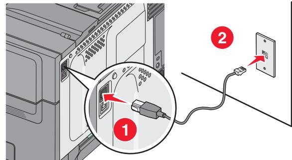
Connect the network cable to the printer and then the wall outlet.
