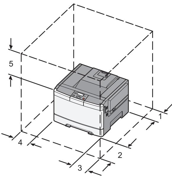
When the printer is set up, allow clearance around it as shown.
