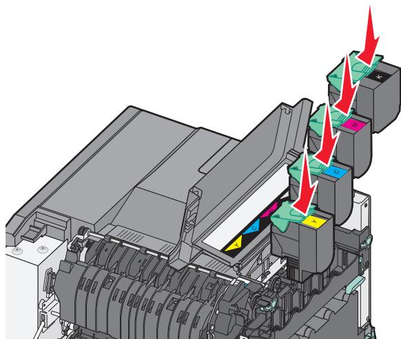
Align and insert the cartridges, and then press down to lock the cartridge.
