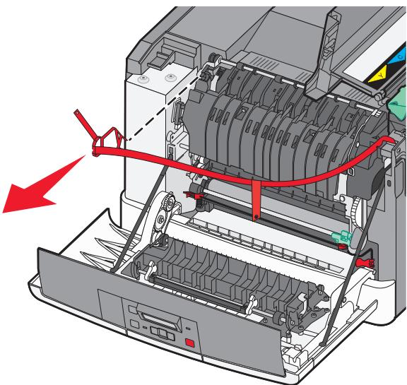
Remove the red packing material.
